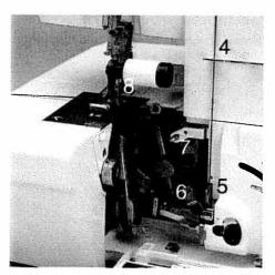
Insert the thread along the path marked in pink through guides 4 to 7.
