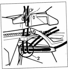
If the looper threads break, you must pull the needle threads out of the needle, rethread the looper threads and then rethread the needle threads.
