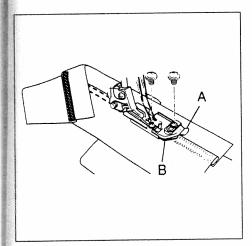
Place the fabric, top side up, under the presser foot, so that the seam on the underside faces the left. The crease of the seam should lie in the inner edge of guide A, adjust guide A as required. On completion of sewing remove guides A and B.
