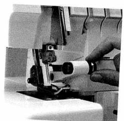
Turn the head of the upper blade away from you until the upper blade locks into a horizontal position.
