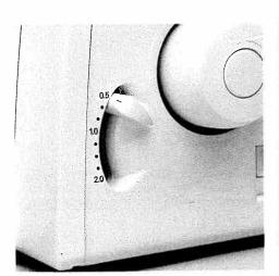
If differential feed adjustment lever (34) is set to 0.5, the front feed dog moves half as fast as the rear feed dog, i.e. the front feed dog feeds through only half as much fabric as the rear feed dog.
