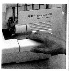
Apply pressure to the lower part of the container until the lower latches click into place in the lower slots of the looper cover.
