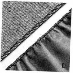
This prevents the seam from becoming stretched when sewing knitted fabrics such as Jersey and rib stitch goods. The result is a smooth seam (C).
