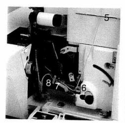
Insert the thread along the path marked in **yellow** through thread guides **5 to 8**.
