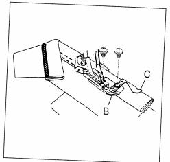
Adjust guide  ${\bf C}$  according to the width of the binding.
