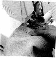
After the second "click" turn the handwheel back, until the needles are in the highest position. Raise the presser foot. Cut the threads. Pull the needle threads to the back and knot them. Hold the threads at the end of the fabric tightly and remove the fabric.
