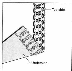
The **lower looper thread** (yellow) appears on the top side of the material.
