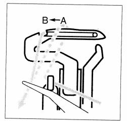
Lay the thread from back to front over the right-hand side of the looper. Carefully pull the thread to the left and slightly down until it slips into notch **B** (= threading point **10**) of the looper.
