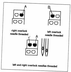
In this instruction manual the various needle positions are shown in a schematic drawing of the needle holder. See the examples above.
