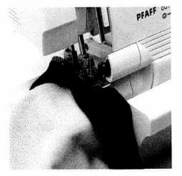
The free arm is particularly useful for sewing tubular items such as trouser legs and sleeves. Insert the article over the free arm.
