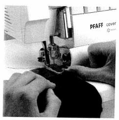
Once a thread chain has been created, the presser foot lifter no longer needs to be raised if you continue working with the same thread and presser foot. It is sufficient to gently lift the presser foot using your thumb. Now slide the fabric under the raised part of the presser foot. The fabric is automatically taken up and fed into the machine when you activate the foot control.
