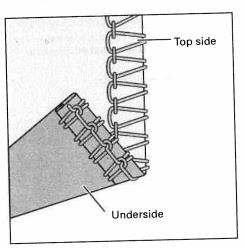
The **right needle thread** (green) is too loose. Set the green thread tension to a higher value and/or the yellow thread tension to a lower value.
