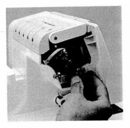
Push the light bulb fully into its socket. Rotate anti-clockwise through half a turn and remove.
