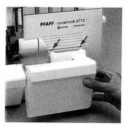
Trimming waste container Insert the upper latches of the trimming waste container (38) into the upper slot of the hook cover (8).
