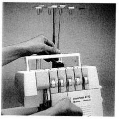
Lift carrying handle (3). Insert the threads beneath the handle and through rear thread guides (37) by pulling down with both hands until the thread slips under the thread guide. Pull the thread between the tension discs and press it down until it is lodged between the tension discs. Return the carrying handle to its closed position.
