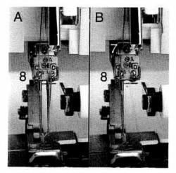
To sew the cover stitch, thread, as shown in illustration **A**, into thread guide **8**. To sew the 2-thread chainstitch, the 5-thread safety-stitch seam and the 4-thread safety stitch seam, thread into thread guides 7 and 8, as shown in illustration **B**. Pull about four inches (10 cm) of thread through the eye of the needle and lay it to the left underneath the presser foot.
