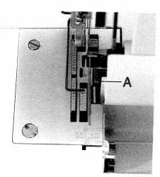
Stitch width latch **A** will be pushed backward. All rolled hems and the cover stitch can be sewn with this setting.
