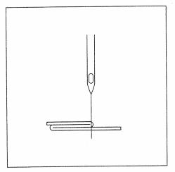
Loosen retaining screw 1 and adjust edge guide 2 so that upon penetration the needle catches only one thread of the upper fabric. Sew a test seam.
