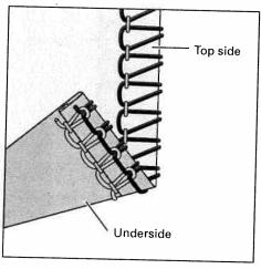
The **right needle thread** (green) is too loose. Set the green thread tension to a higher value.
