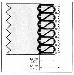
**Note:** The seam width adjustments between 1/8 to 3/16 inch (3.0 mm to 4.5 mm) apply to the right needle only. For the left needle, the set value is increased by 2.2 mm, i.e. the seam width can be continuously adjusted from a scant quarter inch to a generous 1/4 inch (5.2 mm to 6.7 mm).
