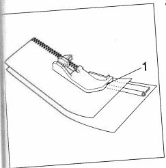
Raise the needle to its uppermost position and insert the cording foot. Place the two fabric plies on top of one another (face side to face side) and insert the cording tape between the two plies. Position the workpiece Working: ween the two plies. Position the workpiece beneath the cording foot ensuring that the cording (piping) runs through groove 1 in the foot.
