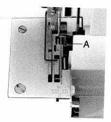
Stitch width latch **A** will be pushed forward. All standard overlock seams can be sewn with this setting.
