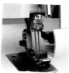
Retaining screw  ${\bf C}$  belongs to the 2-thread chainstitch needle and retaining screw  ${\bf D}$  belongs to the cover-stitch needle.
