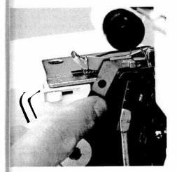
To insert: Insert a new lower blade into the recess provided and tighten the retaining screw. Engage the upper blade and close the looper cover.
