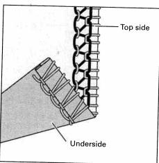
The **lower looper thread** (yellow) is visible on the top side of the fabric.
