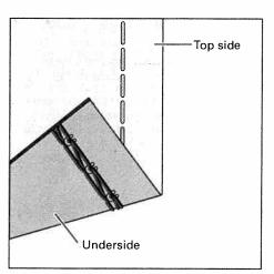
The needle thread (blue) is too loose. Set the blue thread tension to a higher value.
