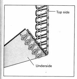
The **left needle thread** (blue) is too loose. Set the blue thread tension to a higher value
