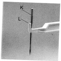
To insert: Insert the needle into the hole of the needle changing aid, so that the flat needle shank (K) faces the flat side (L) of the aid accessory. Now insert the needle fully into the holder and tighten the fastening screw. Remove the needle changing aid. Overlock needle types EL x 705, cat. no. 2002 are required for this machine.
