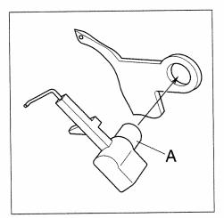
Insert hub **A** of the converter into the aperture of the upper overedge looper.
