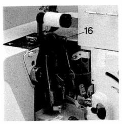
Rotate the handwheel in the direction of the arrow until the upper overedge looper (16) is positioned to the right of the movable upper blade.
