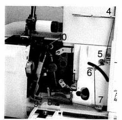
Insert the thread along the path marked in violet through thread guides 4 to 10.
