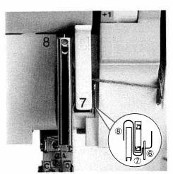
**Note**: The thread must run below the thread guide **7** and above the thread guide **8**.
