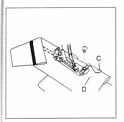
Place the fabric with the top side up under the presser foot. The hemmed seam is in guide **D**, the crease is in guide **C**. Sew the seam and on completion remove guides **C** and **D**.
