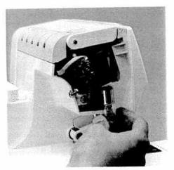
Guide the new light bulb (max. 15 W) into the socket and twist until both pins on the bulb slide into the grooves.
