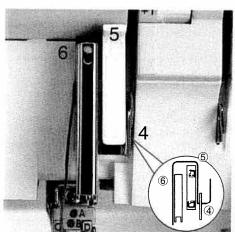
**Note:** The thread must run above thread guides **5 and 6**.
