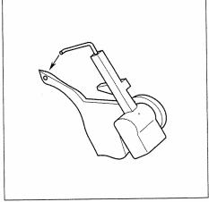
Rotate the converter towards the left and press the upper part slightly to the rear so that the tip of the converter locks into the eye of the looper.
