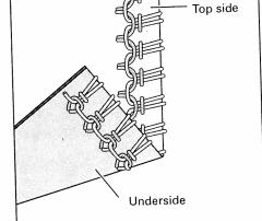
2-Needle, 3-Thread Overedge Closing Seam
