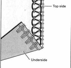
The **upper looper thread** (pink) is visible on the underside of the fabric.
