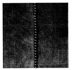
If you wish to sew the beading into the fabric as shown to the left, the needle thread tension must be loose (approx. -5). Lay the material reverse side to reverse side and guide the crease past the upper blade while sewing. Pull the fabric apart; the beading is now on top.
