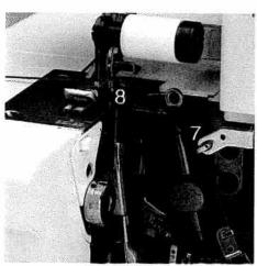
Insert the thread from the front through the eye 8 of the upper overedge looper. Pull about four inches (10 cm) of thread through the looper and lay it to the left underneath the presser foot.
