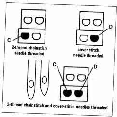
**Note:** If both the 2-thread chainstitch needle and the cover-stitch needle are threaded, the left needle will be somewhat higher than the right needle.
