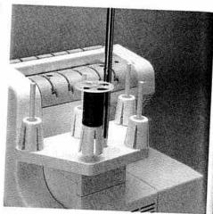
Place the two onto the spool centering piece (30) of the thread spool pin (29).
