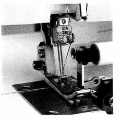
Pull about four inches (10 cm) of thread through the eye of the needle and lay it to the left underneath the presser foot.
