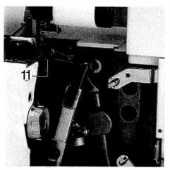
Insert the thread from the front through the eye **11** of 2-thread chainstitch looper.
