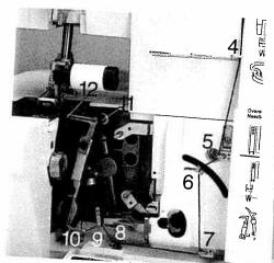
Insert the thread along the path marked in pink through thread guides 4 to 12.
