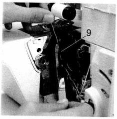
Place the thread, using the tip of the tweezers, into thread guide (9).
