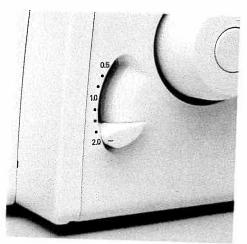
Set differential feed adjustment lever (34) to 2.0 so that the front feed dog moves twice as fast as the rear feed dog, i.e. the front feed dog feeds through twice as much fabric as the rear feed dog.
