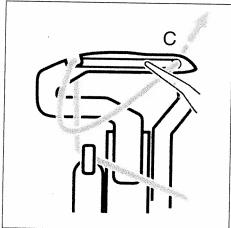
Insert the thread from the front through the eye of lower overedge looper  $\mathbf{C}$  (= threading point 11). The thread must run along the groove in the looper.
