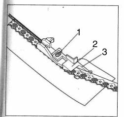
When sewing two lace workpieces together, the two halves must be guided flush along edge guide 3.
