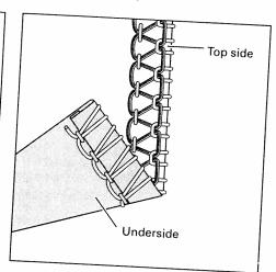
The lower looper thread (yellow) is visible on the top side of the fabric.
